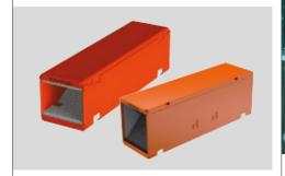
EZ-Path provides you with a fire-safe solution for routing cables through walls and floors. In case of fire, the foam in the EZ-Path will fully expand so that the fire cannot cross over to the next room or floor, etc.
