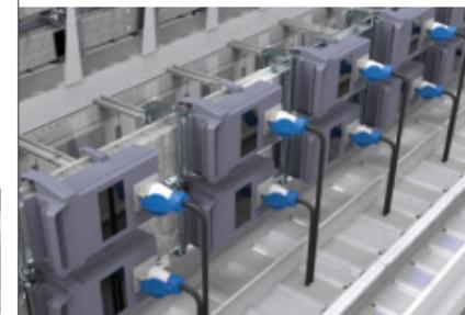
The configuration of the rail conduit system with smart tap-off boxes can be adapted to customer-specific aisle containment layouts in data centres. The system provides a structure for data centre power distribution for power capacities between 160 amperes (A) and 1,000 amperes (A). The system can be easily upgraded if expansion of the existing installation is necessary.
