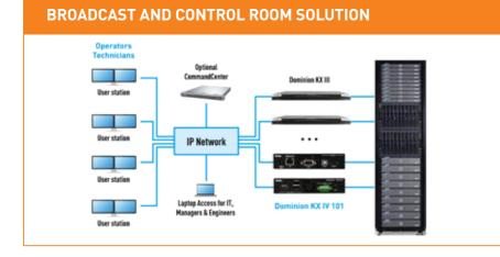
What's more, this switch contains enterprise-level features when it comes to security, flexibility, and has virtual media capabilities that are 3x faster than our previous generation single port KVM-over-IP switch. Another useful feature is the free iOS KVM app allowing the user to configure and administer the KX4-101!"
