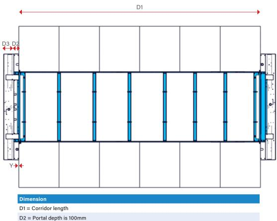
D3 = Sliding door beam depth is 200mm
