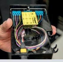
MPO optical fibre cassette, custom made by Legrand. Installation time cut in half in comparison with the old system that was in use.
